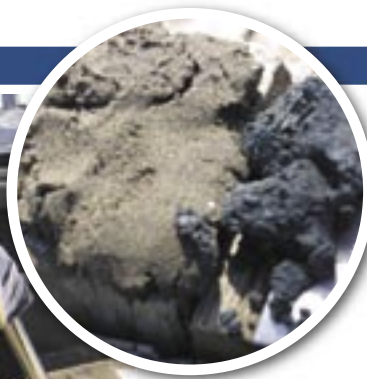
Core samples of the seabed were extracted. A layer of dark sand sat on top of finer, clay-like sand at each of the three locations.
