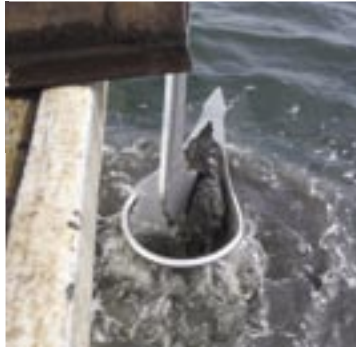
Core samples of the seabed were extracted. A layer of dark sand sat on top of finer, clay-like sand at each of the three locations.
