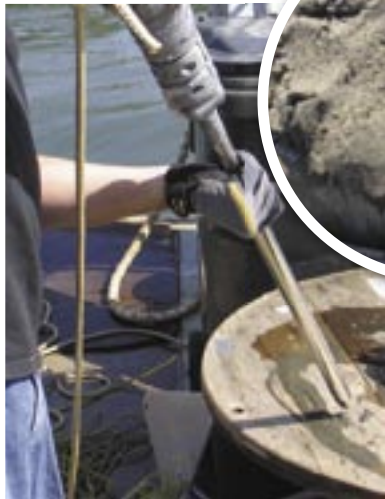
Core samples of the seabed were extracted. A layer of dark sand sat on top of finer, clay-like sand at each of the three locations.
