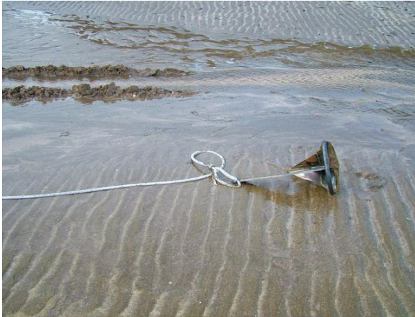
1 These photos demonstrate a standard set in hard sand. Note how the anchor sets itself within its own length. Some scope is simulated by the elevation of the towing vehicle..
