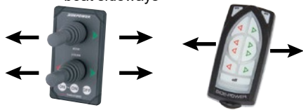
Activating both bow and stern thruster to push the boat sideways
