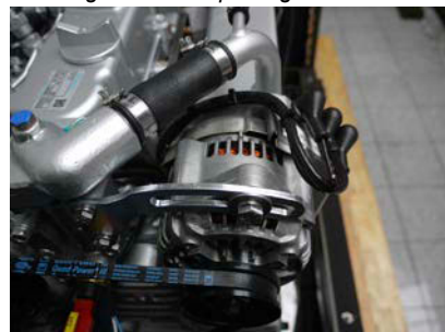
Fig. 8.11-3: Replacing the V-belt
