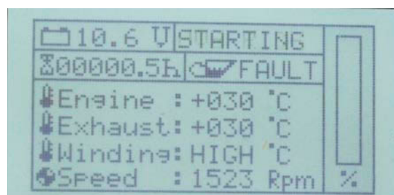
Fig. 16.1.1-2: Warning: „Winding temperature too high“
