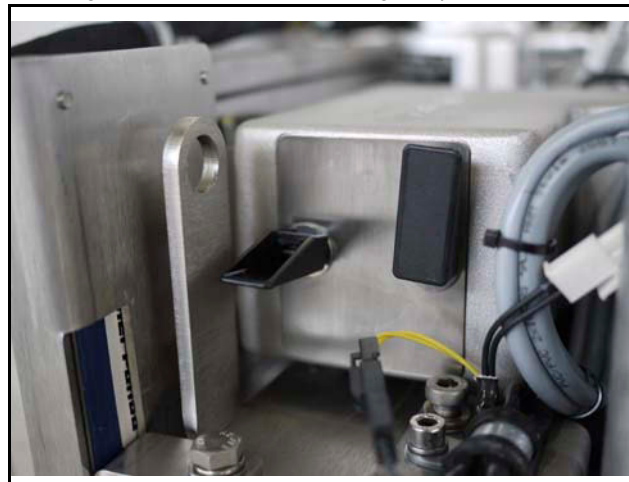
Fig. 10.11.2-2: Air suction housing with pull out holder
