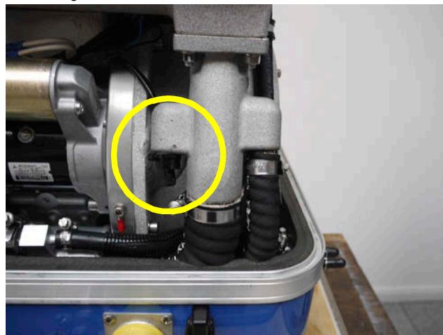
Fig. 7.2.6-2: Thermo-sensor at exhaust connection
