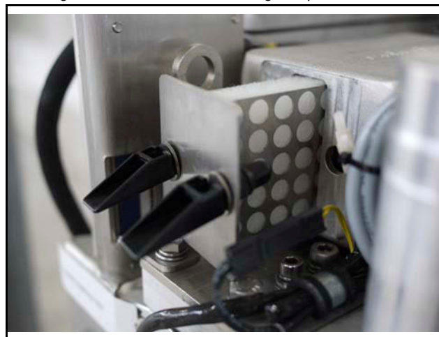
Fig. 10.11.2-3: Air suction housing with pull out holder
