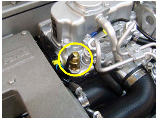
Fig. 7.2.6-1: Thermo.switch at engine
