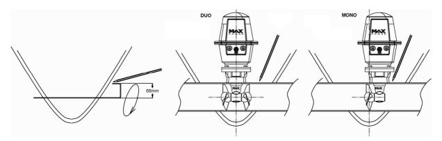
Replace the tunnel. To secure its position apply reinforced fibreglass filler to all areas, both inside and out, taking care to entirely fill the space between the hull and the tunnel. Laminate using a minimum of 8 layers of **ISOPHTALIC RESIN** alternated with mat and roving.
