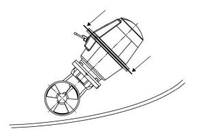
NB: Two metal brackets can be found on the front and back of the casing which can be used to hold the thruster in place if necessary.
