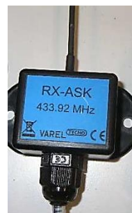
RECEIVING ANTENNA ART. 7CL99017.1 – BES1422 Version "RX-ASK" (433.92 Mhz)
